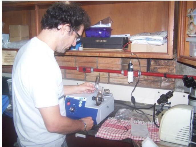
Figure 8 – Cutting a tooth of a manatee in a diamond-embedded blade.
